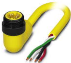
Power cable, 4-position, PVC, yellow, Plug angled 7/8"-16UNF, A - standard, on free cable end, cable length: 1 m
