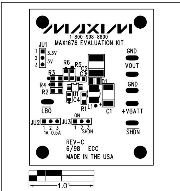
Figure 2. MAX1676 EV Kit Component Placement Guide—Component Side
