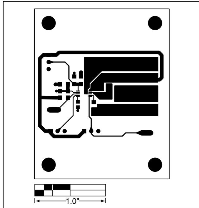
Figure 3. MAX1676 EV Kit PC Board Layout—Component Side
