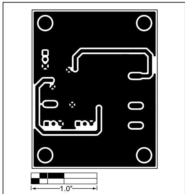
Figure 4. MAX1676 EV Kit PC Board Layout—Solder Side
