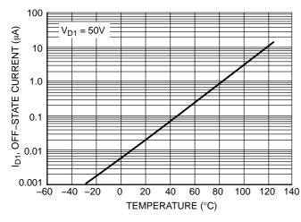
Figure 1. Typical Off-State Current versus Temperature
