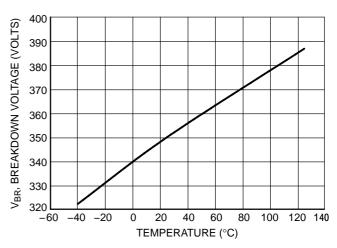
Figure 2. Typical Breakdown Voltage versus Temperature
