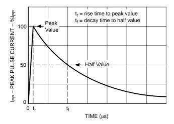
Figure 5. Exponential Decay Pulse Waveform
