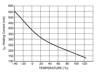
Figure 4. Typical Holding Current versus Temperature
