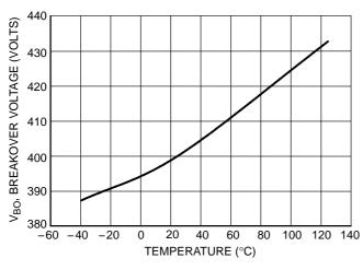
Figure 3. Maximum Breakover Voltage versus Temperature
